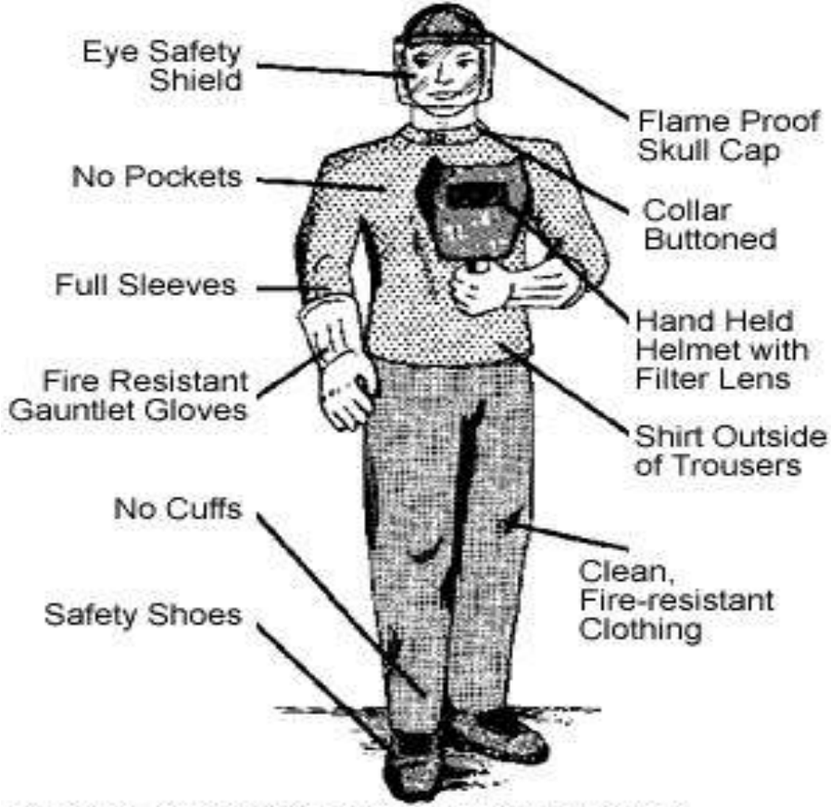
Figure 3. Select clothing to provide maximum protection from sparks and hot metals
